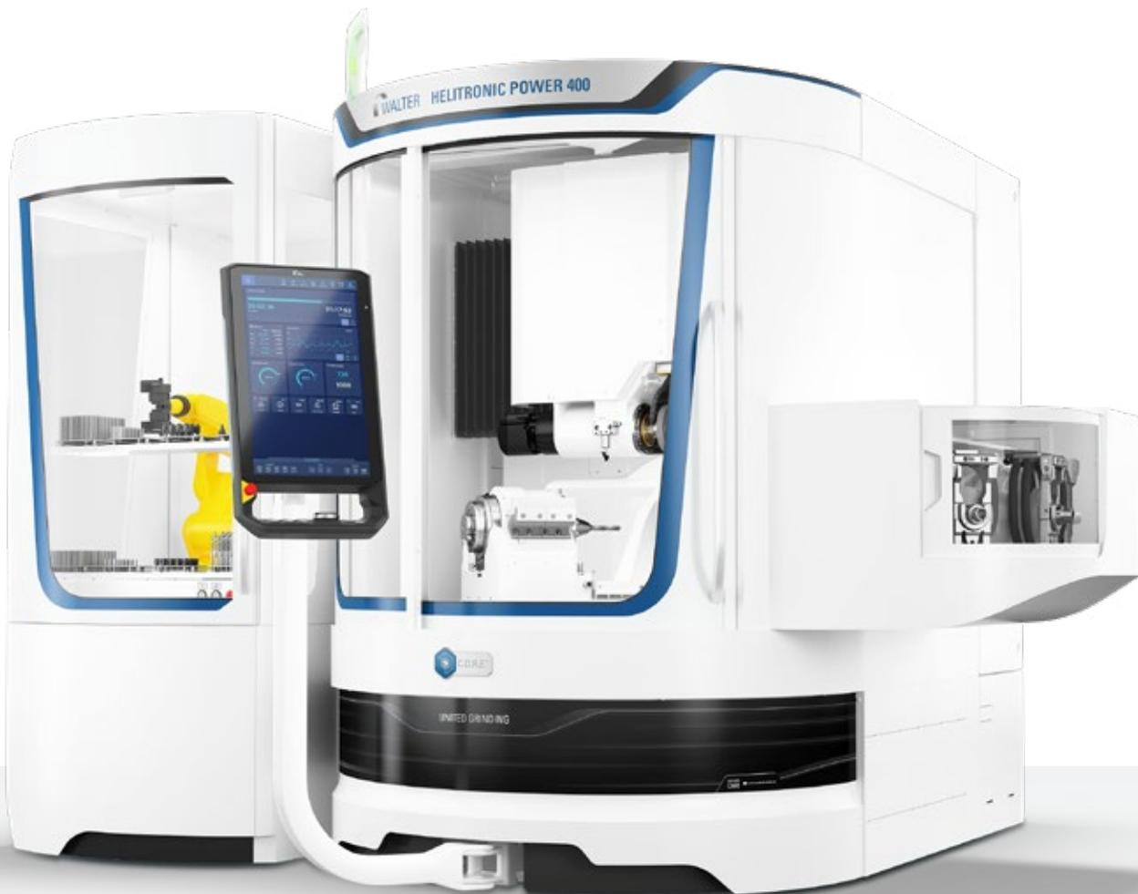
HELITRONIC POWER 400 with the options wheel changer (right) and Robot loader (left)
