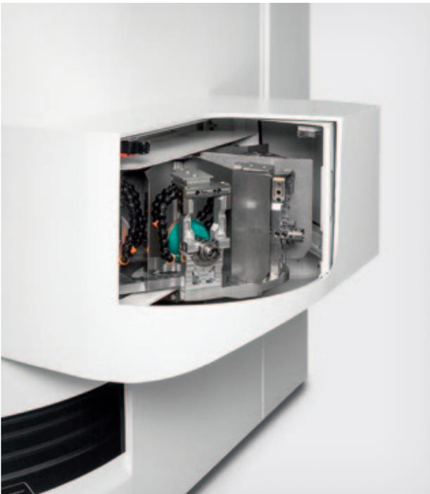
**Directly driven motor spindle (option)**
