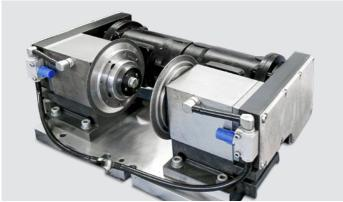
Folding dresser for peripheral, lateral and profile dressing. Pneumatic actuation prevents grinding wheel and grinding wheel guard from colliding with the dresser.
