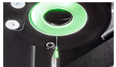
Vertical "90 degree" alignment of the camera
